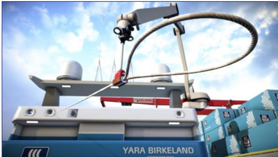
Figure 4: The robotic mooring arm installed on Yara Birkeland Source: MacGregor
